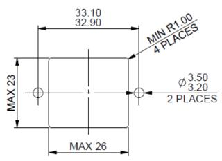
Curtiss Wright recommend the use of 2 x EJOT WN1451-K30-8 screws when utilising the 2 screw mounting points on the centre line. The screws should be tightened to 0.55Nm with a minimum panel thickness of 3 mm. For thicker panels the screw length should be increased to suit.
