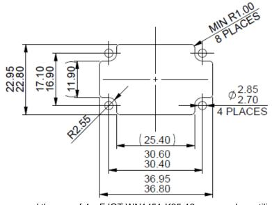
Curtiss Wright recommend the use of 4 x EJOT WN1451-K25-12 screws when utilising the 4 corner screw mounting points. The screws should be tightened to 0.3Nm with a minimum panel thickness of 3 mm. For thicker panels the screw length should be increased to suit.
